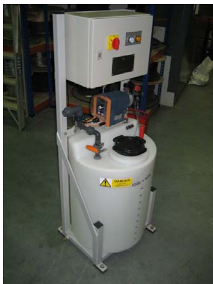
Hypochlorite Dosing Unit
