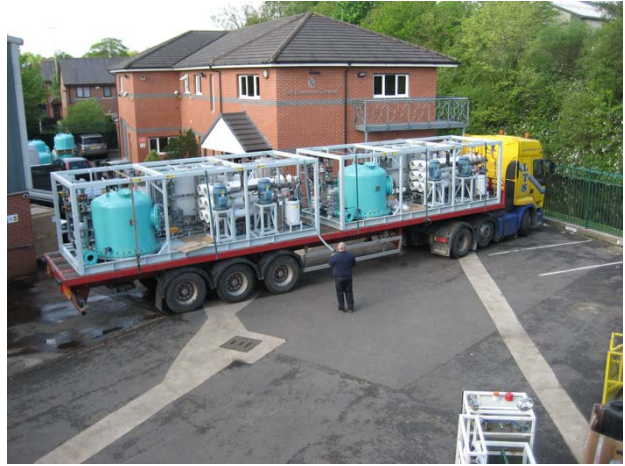
Desalination Plant Being Shipped
