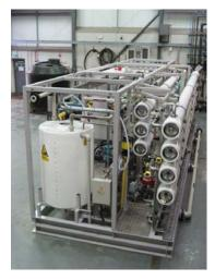
The package is fully self-contained and includes electrical controls, analytical instrumentation (including TOC analyser) and a CIP system.
